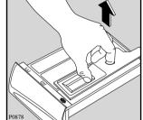
Detergent can also accumulate inside the drawer recess: clean it with an old toothbrush. Refit the drawer after cleaning.
